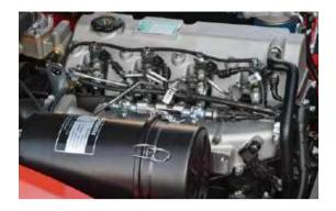
The high pressure common rail electronic-controlled engine which adopts high pressure multiple injections technology to ensure the strong power take-off, lower emission and better cold starting performance; saving the 10% of energy consumption.
