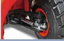
2.0~3.8t roller bearing on the steering axle king pin adopts large size tapered roller bearing (TRB), larger steering cylinder and bumper block assemblies on the top, which can prolong the service life of bearing and highly improve the reliability of steering axle.
